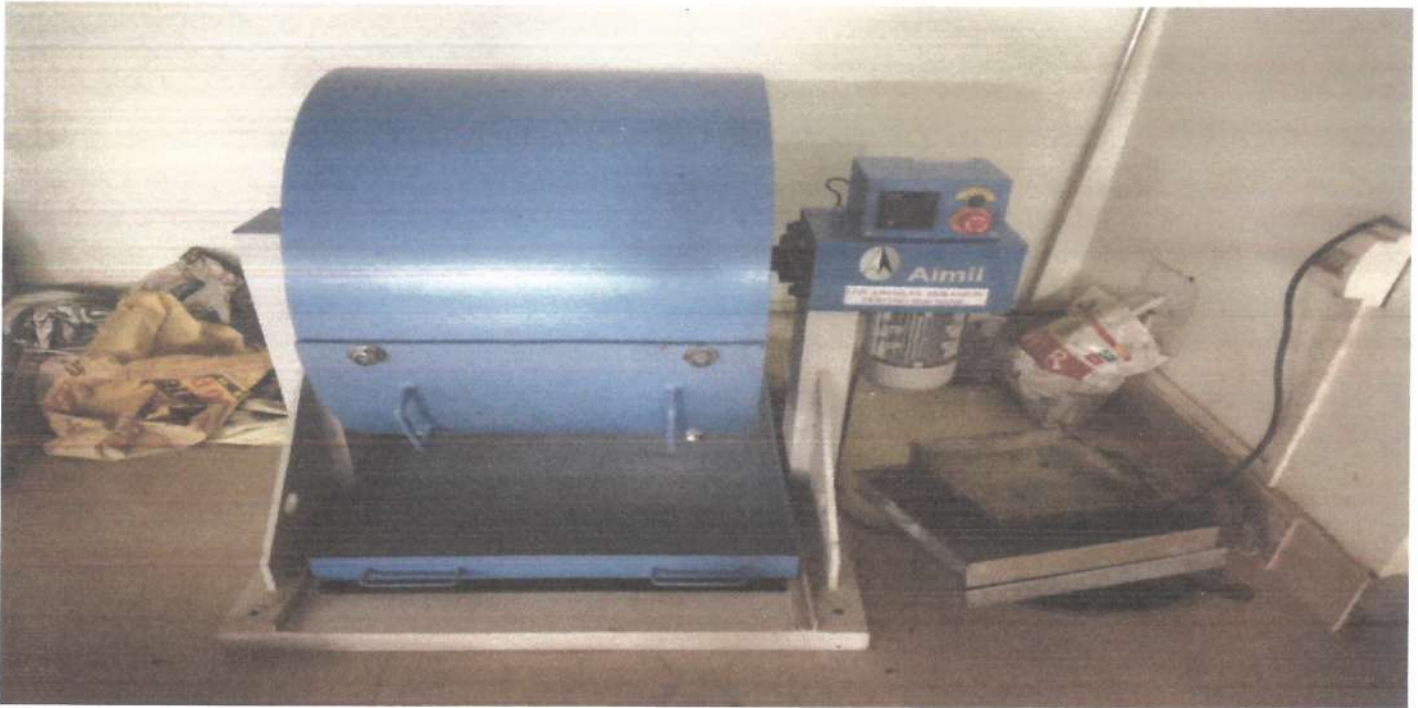
Los Angeles Abrasion Testing apparatus_Transportation Engineering Laboratory_Civil Department
