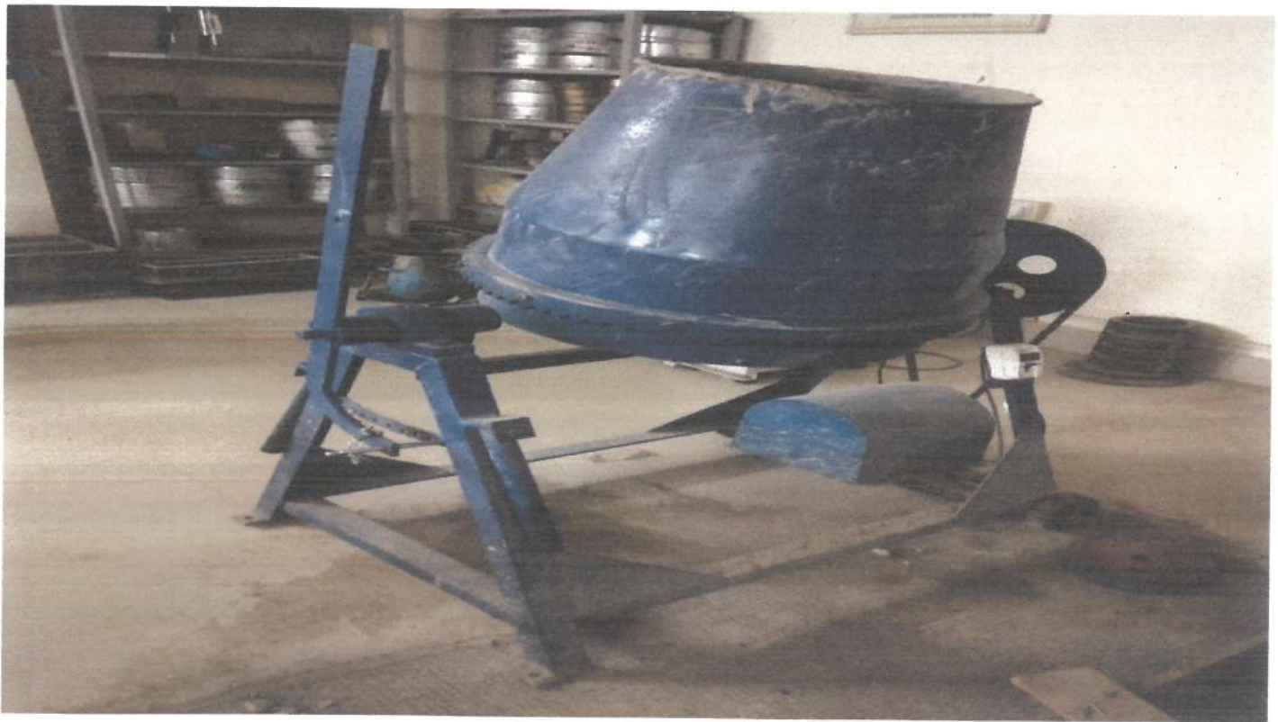
Baby Concrete Mixer 0.5 Cubic Meter_ Concrete Laboratory_ Civil Engg Department
